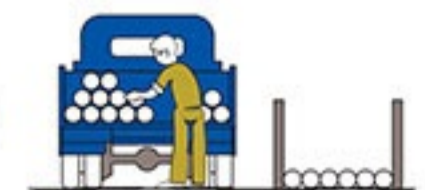
Correct way to off-load pipes
