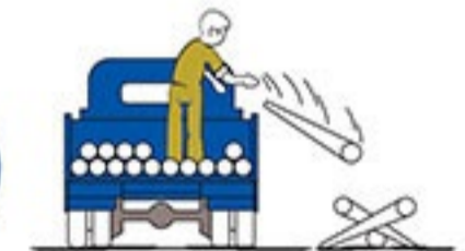
Incorrect way to off-load pipes
